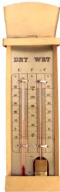
Figure 8.3 Wet and Dry Bulb Thermometer
