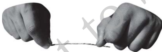
Fig.3.4 Splitting the yarn into thin strands
