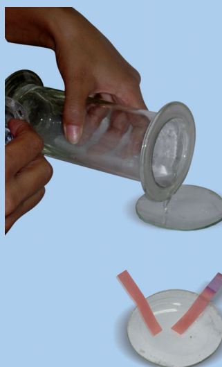
Fig. 4.4 (b) : Testing of solution with litmus papers
